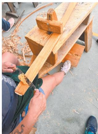
Shaving the excess material to create smooth and attractive splints. Photo by Nate Poyfair.
